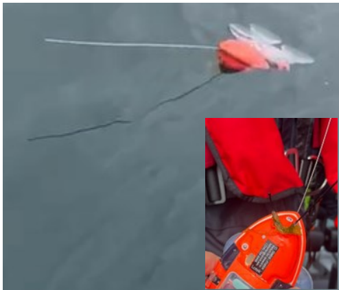
Figure 2. Integrated Dtag floating after deployment mn24_176a. Note the floating angle was such that the ARGOS antennae did not rise above the surface. This was due to some seaweed had become attached to the GPS and ARGOS antennae (inset box). The bad flotation angle explained the relatively low rate of ARGOS positions received (0.37/hr – Table I) when the tag was floating. Photo by Giorgia Giovannini.
