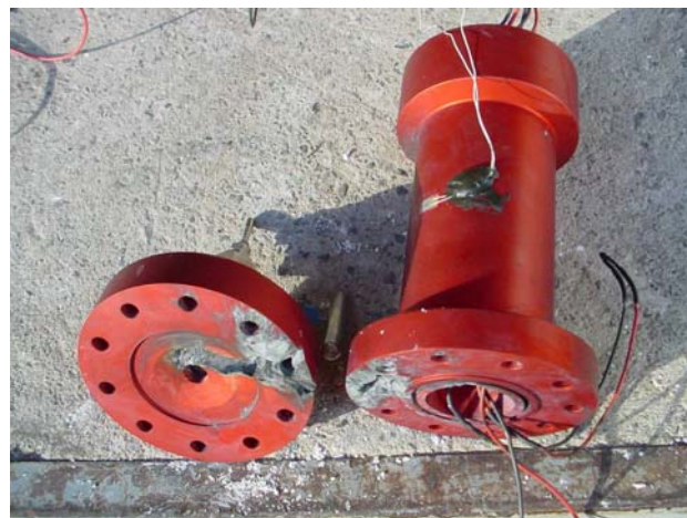
Figure 3. Pressure vessel after pressurizing a cell at 50% SOC with water at a flow of 2 ml/min.
