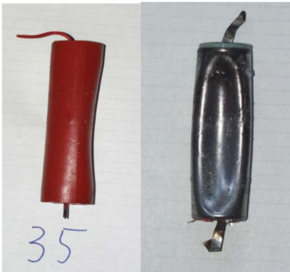
Figure 6. Cell after the experiment in fig 5. Left with potting, right after the removal of the potting.
