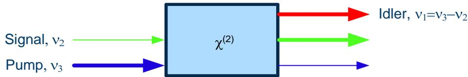
Figure 3.1 Optical parametric amplifier with nonlinear crystal, input beams and output beams. The colours of the beams indicate the relation between the frequencies.
