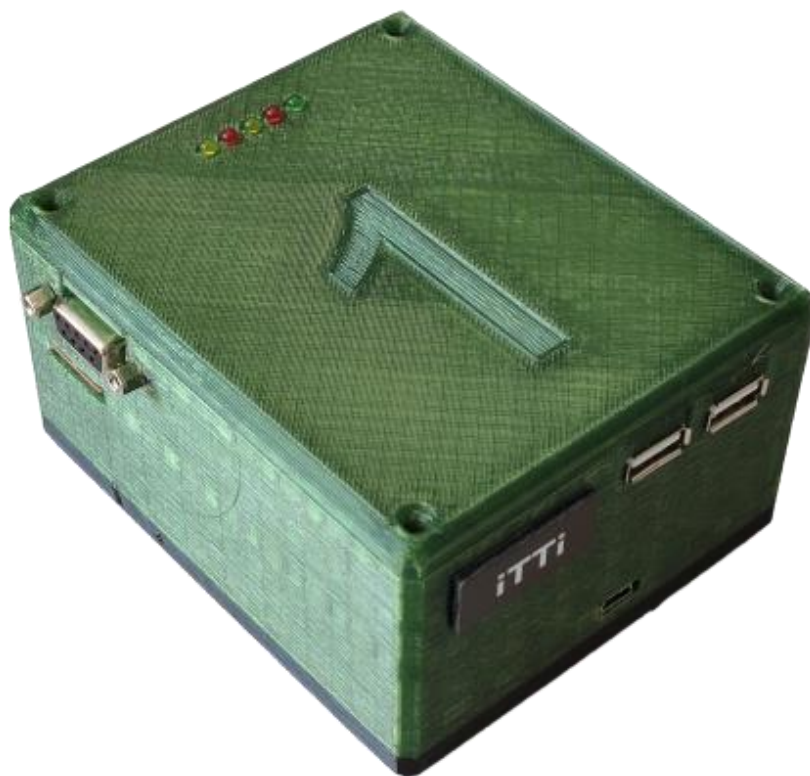
Figure 14 3rd generation of the EU-SENSE sensor node
