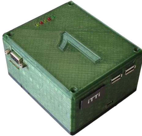
Figure 41 Updated version of the Sensor node (3rd generation)
